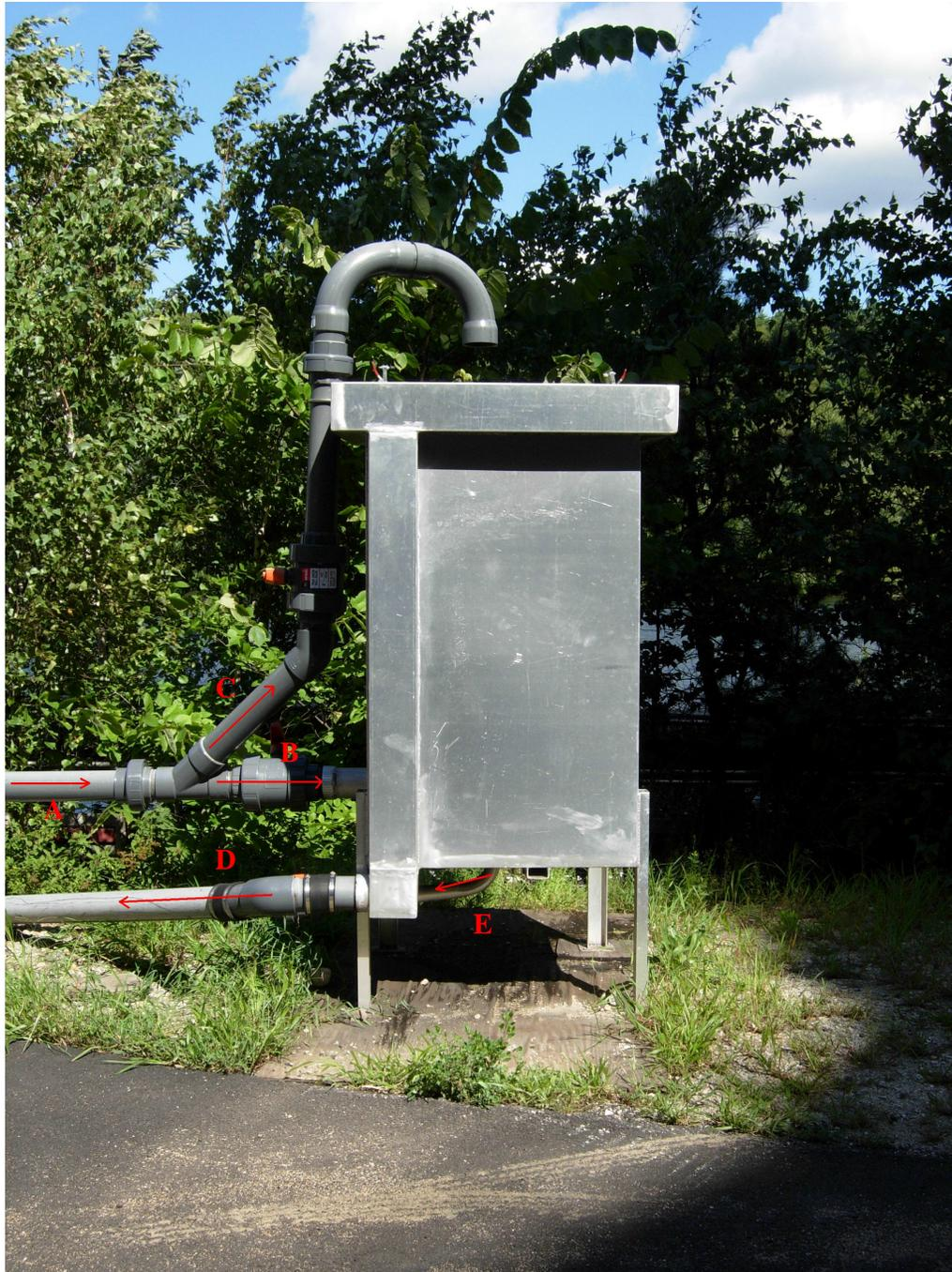
Figure 2-4. Diagram of Merrimack Station entrapment sampler showing flow path through collection tank for entrapment abundance sampling at Unit 1. A: Intake flow to sampling tank, C: Top fill filters down through conical net and sample is collected in cod end, and D: Drain line connected to tank stand pipe. Note: flow path B and E are used for survival sampling and not used for abundance sampling.
