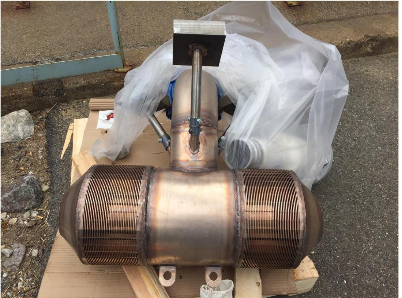
Figure 2-2. T-12 3-mm wedgewire test screen installed in the Merrimack River near the Merrimack Station Unit 1 CWIS. The screen was mounted on a tripod with the six-inch flange below the screen.
