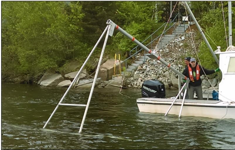
Figure 2-8. Completed assembly (upper photo) and deployment (lower) of the mounting frame used for ADCP data collection in the Merrimack River, NH near the Merrimack Station Unit 1 CWIS during 22 May to 31 August 2017.
